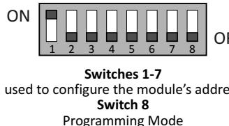
used to configure the module's address
